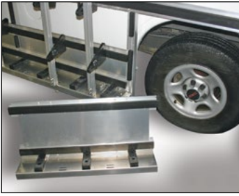
Removable wheel skirt for hassle-free tire changes
