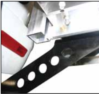
Custom designed, load bearing underbody mounts
