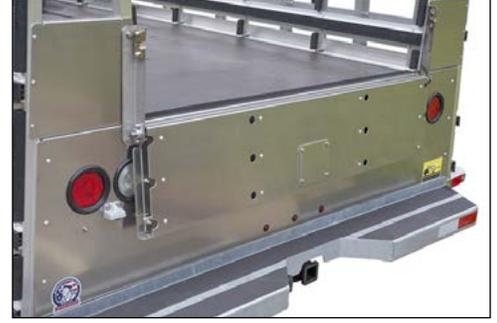
Optional fold-down tailgate and split bumper for hitch receiver
