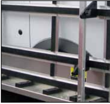
Fixed wheel-skirt and one row of splash panel
