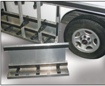
Removable wheel skirt for hassle-free tire changes
